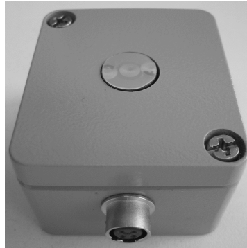
Figure 5.23: Photo from the sensor box with connector and lens from outside
